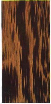
Douglas Fir. Finish 106 B-3 Stained with Bridgeport Standard English Oak Penetrating Stain and Waxed Finish, given a coat of Bridgeport Standard White Shellac, and finished with Bridgeport Standard Prepared Wax.
