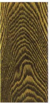
Ash. Finish 3 A-2 Filled with Golden Oak Wheeler's Wood Filler, and finished with Bridgeport Standard Wheeler's Interior Varnish, rubbed egg shell.
