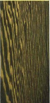
Cypress. Finish 107 D-3 Stained with Bridgeport Standard Flemish Oak Penetrating Stain and Waxed Finish, given a coat of Bridgeport Standard White Shellac, and finished with Bridgeport Standard Prepared Wax.
