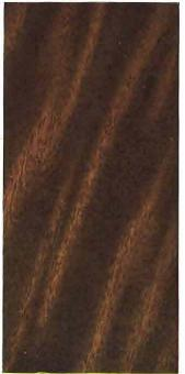
Mahogany. Finish 220 A-2 Stained with Bridgeport Standard No. 3000-A Mahogany Acid Stain, filled with Mahogany "N" Wheeler's Wood Filler, and finished with Bridgeport Standard Wheeler's Interior Varnish, rubbed egg shell.
