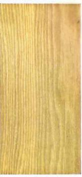
Ash. Finish 1 A-2 Filled with No. 1 Wheeler's Wood Filler, and finished with Bridgeport Standard Wheeler's Interior Varnish rubbed egg shell.
