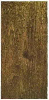
Poplar. Finish 105 D-3 Stained with Bridgeport Standard Brown Oak Penetrating Stain and Waxed Finish, given a coat of Bridgeport Standard White Shellac, and finished with Bridgeport Standard Prepared Wax.
