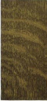
Quartered White Oak, Finish 107 D-3 Stained with Bridgeport Stand-ard Flemish Oak Penetrating Stain and Waxed Finish, given a coat of Bridgeport Standard White Shel-lac, and finished with Bridgeport Standard Prepared Wax.
