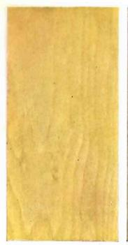
Hemlock. Finish 9 A-1 Given a coat of Bridgeport Standard Wheeler's Silex Liquid Wood Filler, and finished with Bridgeport Standard Wheeler's Bridgeport Standard Wheele Interior Varnish left in the gloss.
