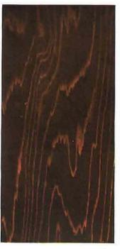
Hemlock. Finish 108 C-5 Hemlock. Finish 108 C-5 Stained with Bridgeport Standard Dark Mahogany Penetrating Stain, given a coat of Bridgeport Standard Mahogany Primer, and finished with one coat of Bridgeport Standard Wheeler's Interior Varnish, and one coat of Bridgeport Standard Wheeler's Flat Varnish.
