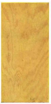
Douglas Fir. Finish 8 B-1 Given a coat of Bridgeport Standard Wheeler's Liquid Wood Filler and finished with Bridgeport Standard Wheeler's Interior Varnish, left in the gloss.
