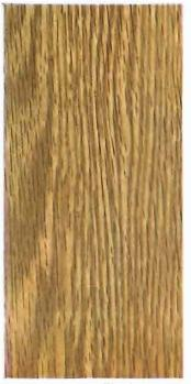
Plain Red Oak. Finish 1 A-2 Filled with No. 1 Wheeler's Wood Filler and finished with Bridgeport Standard Wheeler's Interior Varnish, rubbed egg shell.
