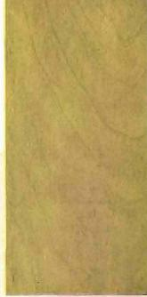
Plain Red Gum. Finish 1 A-2 Filled with No. 1 Wheeler's Wood Filler, and finished with Bridgeport Standard Wheeler's Interior Varnish, rubbed egg shell.
