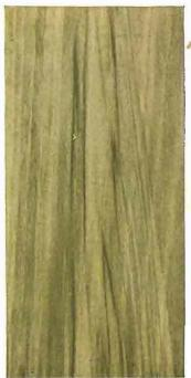
Quartered Red Gum. Finish 114 D-3 Stained with Bridgeport Standard No. 2303 Circassian Walnut, Penetrating Stain, given a coat of Bridgeport Standard White Shellac, and finished with Bridgeport Standard Prepared Wax.
