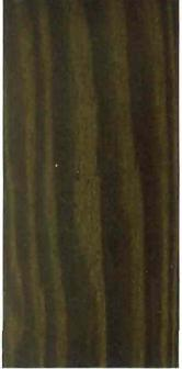
California Redwood. Finish 110 D-3 Stained with Bridgeport Stand-ard 530 Mission Green Penetrating Stain, given a coat of Bridgeport Standard White Shellac, and fin-ished with Bridgeport Standard Prepared Wax.
