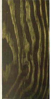
North Carolina Pine. Finish 106 D-3 Stained with Bridgeport Stand-ard Flemish Oak Penetrating Stain and Waxed Finish, given a coat of Bridgeport Standard White Shellac, and finished with Bridgeport Stand-ard Prepared Wax. ard Prepared Wax.
