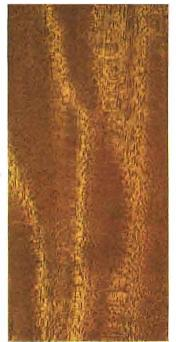
Mahogany. Finish 7 A-2 Filled with No. 7 Wheeler's Wood Filler, and finished with Bridgeport Standard Wheeler's Interior Varnish, rubbed egg shell.
