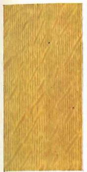
Quartered White Oak. Finish I A-2 Filled with No. 1 Wheeler's Wood Filler, and finished with Bridgeport Standard Wheeler's Interior Varnish, rubbed egg shell.
