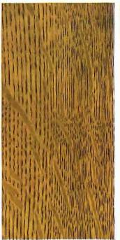
Quartered White Oak. Finish 2 A-2 Filled with No. 3 Wheeler's Wood Filler, and finished with Bridgeport Standard Wheeler's Interior Varnish, rubbed egg shell.
