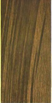
Quartered Red Gum. Finish 113 C-2 Stained with Bridgeport Standard No. 2090 Light Mahogany Penetrating Stain, given a coat of B.S. Mahogany Primer, and finished with B. S. Wheeler's Interior Varnish, rubbed egg shell.
