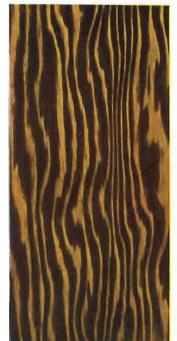
Douglas Fir. Finish 112 D-3 Stained with Bridgeport Standard R. Y. Golden Oak Penetrating Stain, given a coat of Bridgeport Standard White Shellac, and finished with Bridgeport Standard Prepared Wax.
