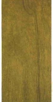
Cherry. Finish 1 A-2 Filled with No. 1 Wheeler's Wood Filler, and finished with Bridgeport Standard Wheeler's Interior Varnish, rubbed egg shell.
