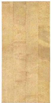
Maple Flooring. Finish 1 J-1 Filled with No. 1 Wheeler's Wood Filler, and finished with Bridgeport Standard Wheeler's Floor Varnish.
