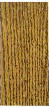
Plain Red Oak. Finish 2 A-2 Filled with No. 3 Wheeler's Wood Filler, and finished with Bridgeport Standard Wheeler's Interior Varnish, rubbed egg shell.
