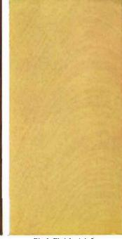
Birch Finish 1 A-2 Filled with No. 1 Wheeler's Wood Filler, and finished with Bridgeport Standard Wheeler's Interior Varnish, rubbed eggshell.
