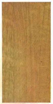
Quartered White Oak Flooring Finish 1 J-1 Filled with No. 1 Wheeler's Wood Filler, and finished with Bridgeport Standard Wheeler's Floor Varnish.
