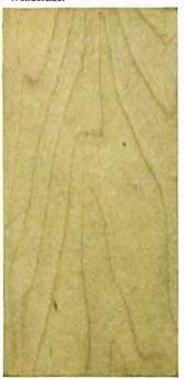
Maple, Finish 1 A-2 Filled with No. 1 Wheeler's Wood Filler, and finished with Bridgeport Standard Wheeler's Interior Varnish, rubbed egg shell.
