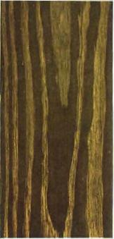
Southern Yellow Pine. Finish 107 D-3 Stained with Bridgeport Stand-ard Flemish Oak Penetrating Stain and Waxed Finish, given a coat of Bridgeport Standard White Shel-lac, and finished with Bridgeport Standard Prepared Wax.
