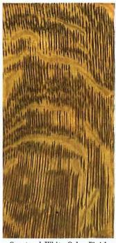
Quartered White Oak. Finish 116 A-2 Stained with Bridgeport Standard R. Y. Golden Oak Penetrating Stain, filled with No. 3 Wheeler's Wood Filler, and finished with Bridgeport Standard Wheeler's Interior Varnish, rubbed egg shell.
