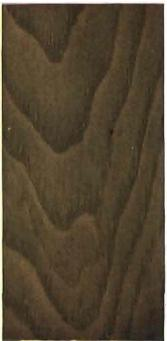
Plain Red Gum. Finish 108 C-5 Stained with Bridgeport Standard Dark Mahogany Penetrating Stain, given a coat of Bridgeport Standard Mahogany Primer, and finished with one coat of Bridgeport Standard Wheeler's Interior Varnish, and one coat of Bridgeport Standard Wheeler's Flat Varnish.
