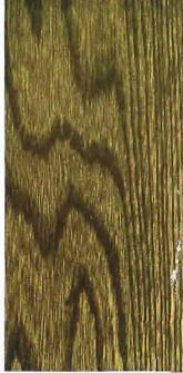
Elm. Finish 3 A-2 Filled with Golden Oak Wheeler's Filled with Golden Oak Wheeler's Bridgeport Standard Wheeler's Interior Varnish, rubbed egg shell.
