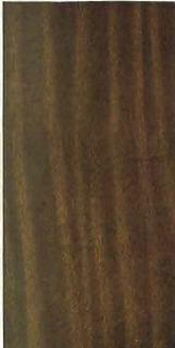
Mahogany, Finish 218 A-2 Stained with Bridgeport Standard No. 1 Standard Brown Mahogany Acid Stain, filled with No. 16 Brown Mahogany Wheeler's Wood Filler, and finished with Bridgeport Standard Wheeler's Interior Varnish, rubbed egg shell.
