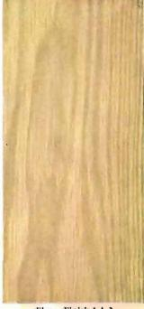
Elm. Finish 1 A-2 Filled with No. 1 Wheeler's Wood Filler, and finished with Bridgeport Standard Wheeler's Interior Varnish, rubbed egg shell.
