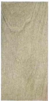
Tupelo. Finish 224 E-1 Stained with Bridgenort Standard Gray Acid Stain, given a coat of Bridgeport Standard No 3001 Smoked Pearl Toner, and finished with two coats of Bridgeport Standard WonderLac.
