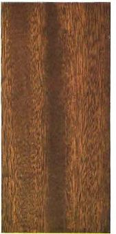
Mahogany. Finish 219 A-2 Stained with Bridgeport Standard No. 5 Sheraton Mahogany Acid Stain, filled with No. 18 Sheraton Mahogany Wheeler's Wood Filler, and finished with Bridgeport Standard Wheeler's Interior Varnish, rubbed egg shell.
