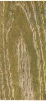
Chestnut. Finish 212 H-1 Stained with Bridgeport Standard Gray Acid Stain, filled with Special White Wheeler's Wood Filler, and finished with Bridgeport Standard Prepared Wax.
