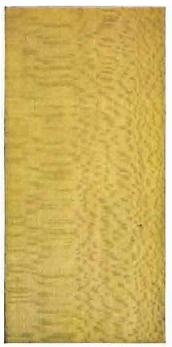
Sycamore. Finish 1 A-2 Filled with No. 1 Wheeler's Wood Filler, and finished with Bridgeport Standard Wheeler's Interior Varnish, rubbed egg shell.
