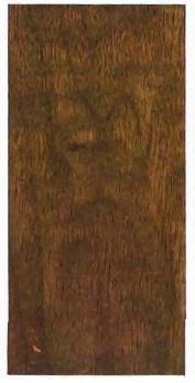
American Walnut. Finish 2 A-2 Filled with No. 3 Wheeler's Wood Filler, and finished with Bridgeport Standard Wheeler's Interior Varnish, rubbed egg shell.
