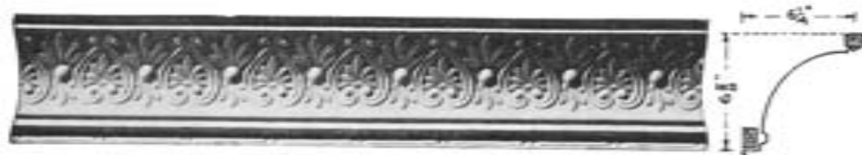
No. 4816 Cornice 6 \frac{1}{4} in. projection 6 \frac{3}{4} in. deep 48 in. long 10 cents per lineal foot (without brackets) 11 cents per lineal foot (with brackets)
