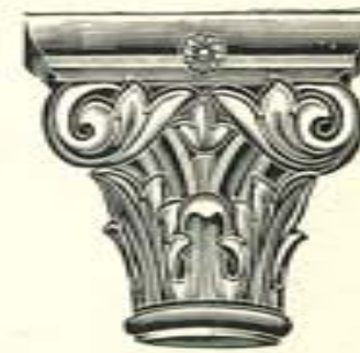
No. 1658. Diameter at neck, 5 in.; height, 11½ in.; width at abacus, 13 in. Full Capital, in parts, each, $8.50.
