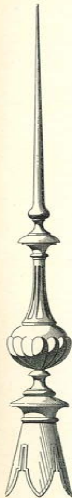
No. 2059. Stem of Wrought Iron Pipe. Height, 8 feet.
